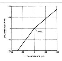
Figure 17. Typical  $\Delta$  Output Delay vs.  $\Delta$  Capacitance (pF)
